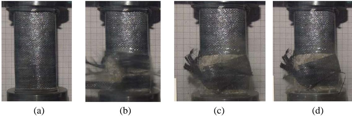
Fig. 6. Progressive failure of a brick aggregate concrete CFRP-confined column (150 mm x 150 mm x 300 mm) under axial compression captured from high-definition video footage. The side opposite to the lap is facing the camera. Locations of the captured still image frames in the HD footage: (a) 2 min : 13 sec : 58/60 frame, (b) 2 min : 14 sec : 01/60 frame, (c) 2 min : 14 sec : 10/60 frame, (d) 2 min : 14 sec : 18/60 frame. Images by A.F.M.S. Amin.
