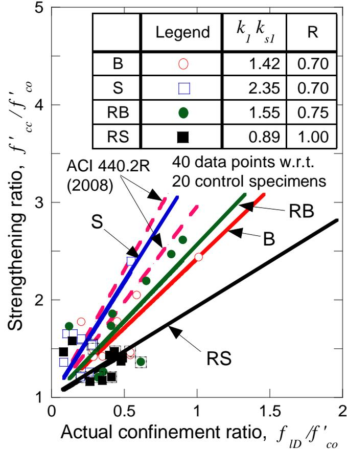
Fig. 10. Strengthening ratio vs. actual confinement ratio plots for CFRP-confined and GFRP-confined columns. Data points inside the dotted box are derived from the dataset presented in Figures 8 and 9.
