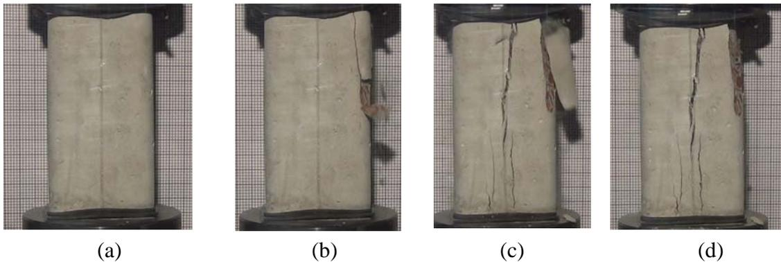
Fig. 5. Progressive failure of brick aggregate concrete control column (150 mm x 150 mm x 300 mm) under axial compression captured from high-definition video footage. Locations of the captured still image frames in the HD footage: (a) 1 min : 53 sec : 20/60 frame, (b) 1 min : 53 sec : 30/60 frame, (c) 1 min : 54 sec : 37/60 frame, (d) 1 min : 55 sec : 00/60 frame. Images by A.F.M.S. Amin.
