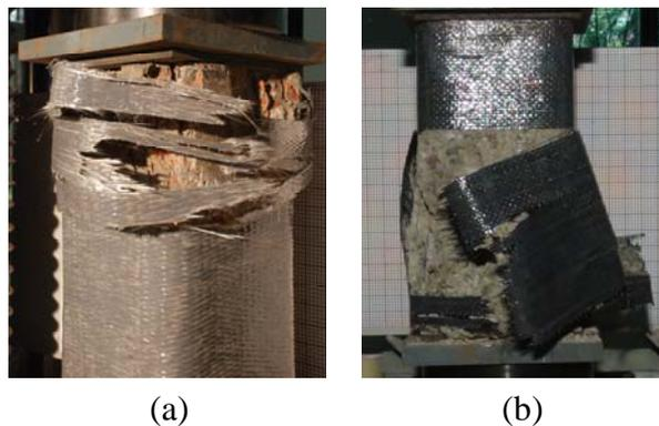
Fig. 7. Failure patterns of FRP-confined 200 mm x 200 mm x 400 mm columns. After the end of the tests, the specimens were rotated to get the best view of the failure location. (a) GFRP rupture in confined brick aggregate concrete column, (b) CFRP rupture in confined recycled stone aggregate concrete column. Images by A.F.M.S. Amin.
