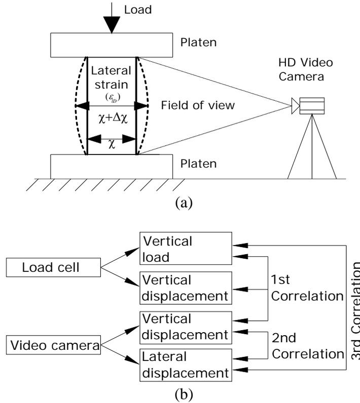
Fig. 4. DICT to measure lateral strain. (a) Layout of the test apparatus (b) Data acquisition scheme. Lateral strain,  $\varepsilon_{D} (= \Delta\chi/\chi)$ , is taken as an indirect measure of the dilation effect, where  $\chi$  is the initial width of the specimen and  $\Delta\chi$  is the increase in width due to dilation.
