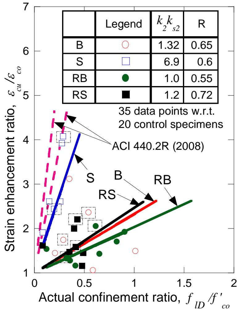
Fig. 11. Strain enhancement ratio vs. actual confinement ratio plots for CFRP-confined and GFRP-confined columns. Data points inside the dotted box are derived from the dataset presented in Figures 8 and 9.
