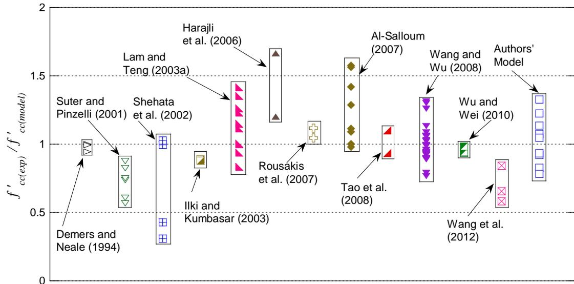
Fig. 12. Representation of confined compressive strengths against different published test data sets on stone aggregate concrete square columns by Authors' model using the  $k_1 k_{s1}$  coefficient of Equation 1 assessed in Figure 10.  $f'_{cc(\text{exp})}$  are the test data taken from different published studies, and  $f'_{cc(\text{model})}$  are respective predicted confined compressive strengths obtained using the authors' model.
