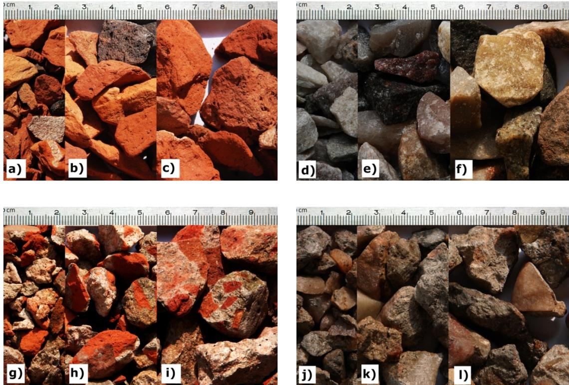
Fig. 3. Types of coarse aggregates used in the research (a), (b), (c) are brick aggregates, (d), (e), (f) are stone aggregates, (g), (h), (i) are recycled brick aggregates and (j), (k), (l) are recycled stone aggregates. Here, (a), (d), (g), (j) aggregates are of 12 mm passing and 6.3 mm retained; (b), (e), (h), (k) are of 19 mm passing and 12 mm retained, and (c), (f), (i), (l) are of 25 mm passing and 19 mm retained. Images by A.F.M.S. Amin.
